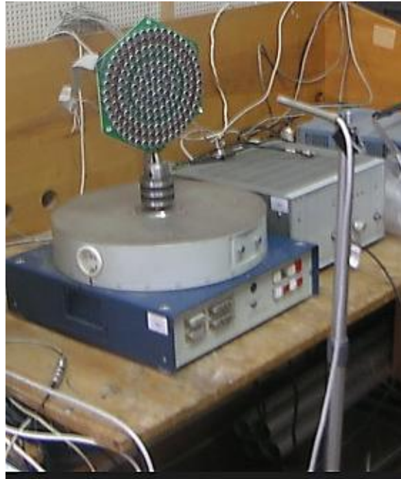
Fig. 8. Installation for measuring the ultrasonic field.
