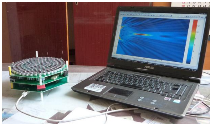
Fig. 7. Ultrasonic matrix and control computer
