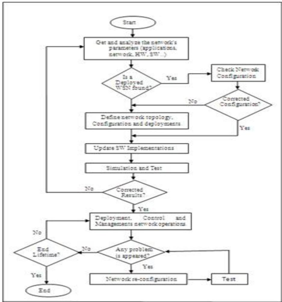
**Fig. (2): Flow chart of the proposed system Operation**
